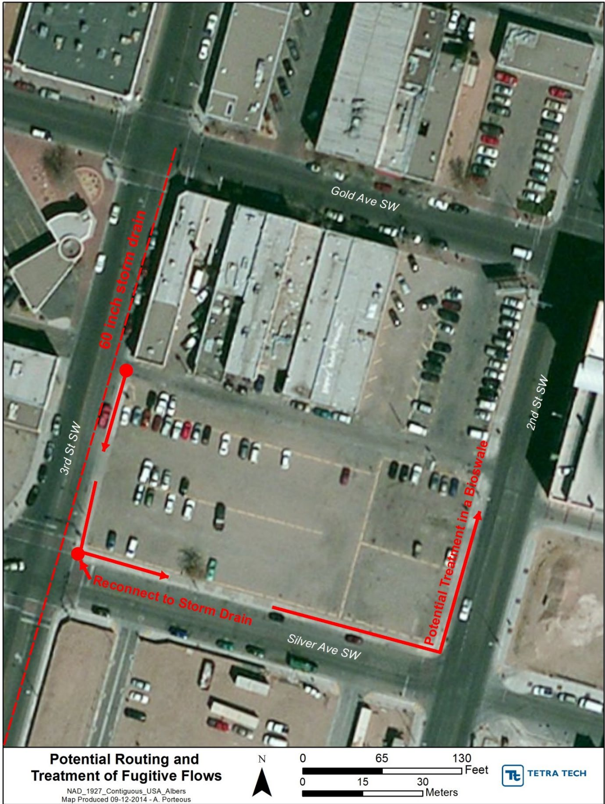
Figure 3-3. Potential routing and treatment of fugitive flows.
