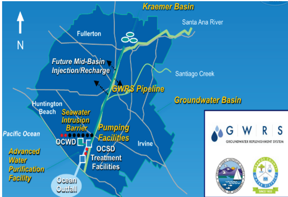
Figure A.2-2. Map of GWRS facilities, pipeline and recharge basins (Source: GWRS)
