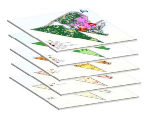
The figure above is a visual representation of the overlaying of land use, soil, slope, imperviousness, and structure layers to create a single HRU layer for Tisbury, MA.
