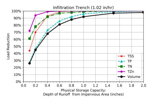
This Performance Curve is for an Infiltration Trench SCM. At a design storage volume (DSV) sizing of 0.4 in. of runoff depth, a practitioner can expect to control better than 90% of the nitrogen load from the contributing impervious cover (IC) areas. The represents DSV the maximum design volume storage capacity of a SCM to hold water (i.e., equals volume of potential
