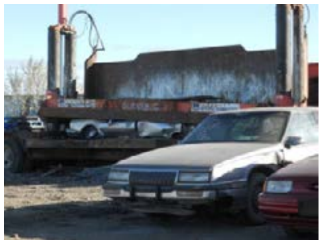
Vehicle Crusher in Operation
