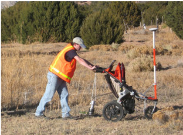
Contractors, along with EPA and NNEPA, evaluating a yard with radiation-specific instruments and survey equipment. It takes about three hours to evaluate inside and outside the home.
