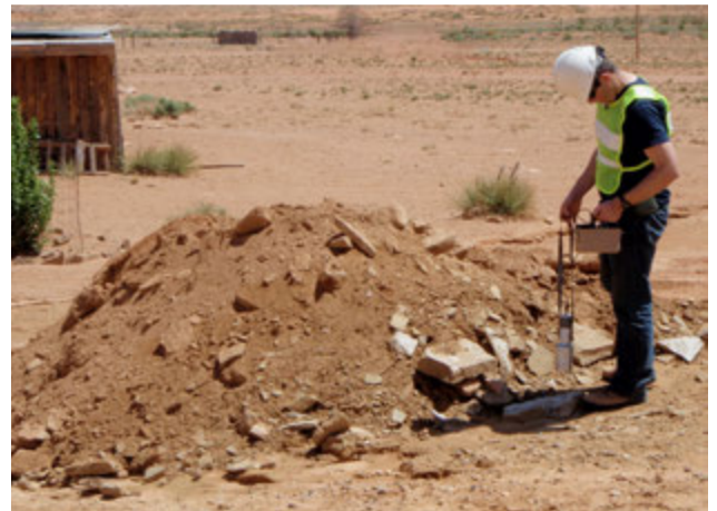
Contractors, along with EPA and NNEPA, evaluating a yard with radiation-specific instruments and survey equipment. It takes about three hours to evaluate inside and outside the home.
