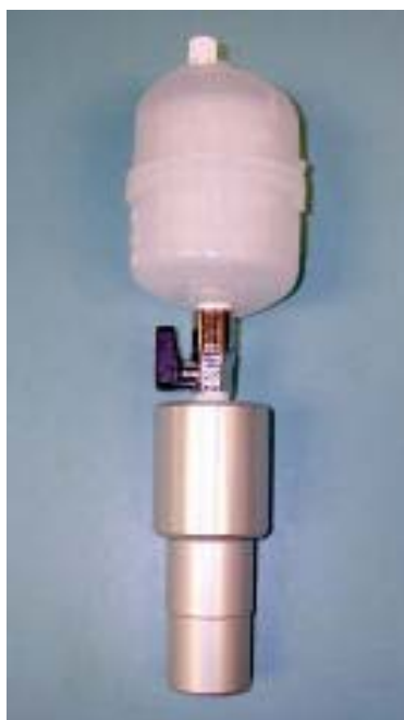
Figure 9-14. The BX-302 Zero Calibration Kit is required for the BKGD zero test.
