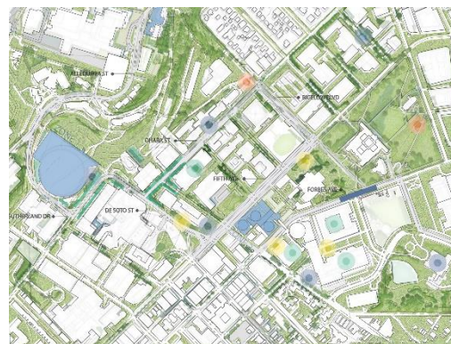
Figure 11: Campus Masterplan adaptations red - rain garden, Black - Bioswale, Green - Green roof, and Yellow - Pervious Surface.
