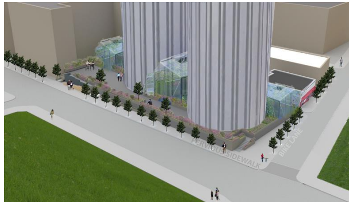
Figure 14: Towers Plaza Green Atrium proposed site rendering. Sloped glass roofing, edible gardens, gray water storage and tree pits will transform this historic residence hall into a sustainable beacon.
