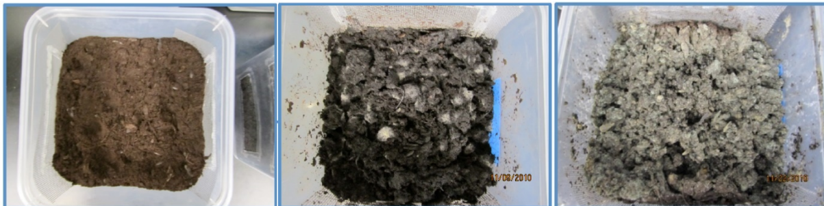
FIGURE 9. INCREASED FUNGAL GROWTH OVER TIME ON DEHYDRATED FOOD WASTE
