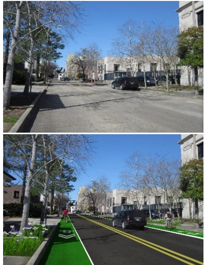
Artistic rendering of a street redesign to include narrower lanes, bike lanes, and planters.
