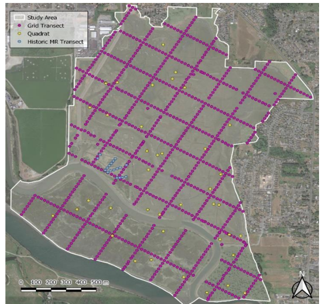
MAP SHOWING GRID POINTS AND TRANSECTS FOR RTK SURVEYS OF SURFACE ELEVATION. FIGURE 17. SNOHOMISH ESTUARY MONITORING
