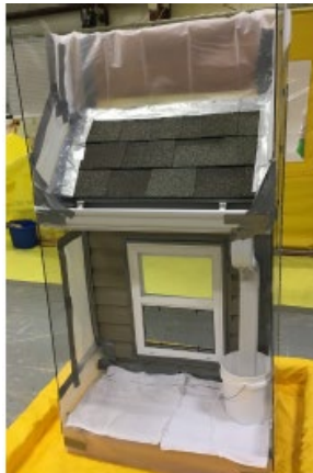
*Mock Wall setup used for spray decontamination experiments of roofing and siding surfaces. In this photo set up with asphalt shingles, vinyl siding, window, gutter, and downspout.
