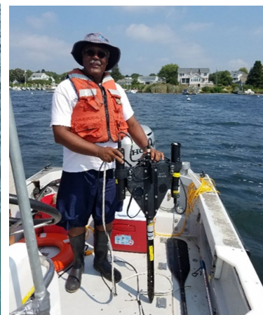
Left: Water quality buoys help researchers measure physical, chemical, and biological properties of water in Shubael and Hamblin Ponds. Right: EPA scientist Darryl Keith with the in-water HyperSAS profiling radiometer system which measures the spectrum of the underwater light field. The HyperSAS spectral signatures will provide in-water validation of remote sensing algorithms to map seagrass density and estimate phytoplankton and cyanobacteria concentrations derived from satellites, aircraft, and UAV data.
