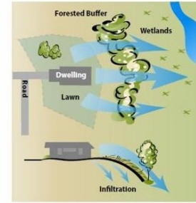
Figure 18. Concept Development CD3.4 LID to Achieve the Watershed Protection Standard for Low Density Residential
