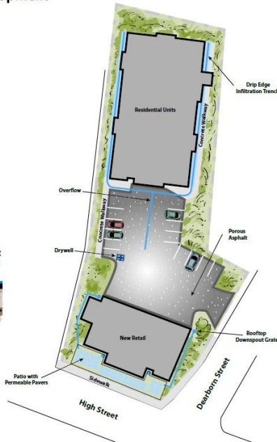
Figure 11. Concept Development CD2.4 LID to Achieve the Watershed Protection Standard for Commercial Redevelopment
