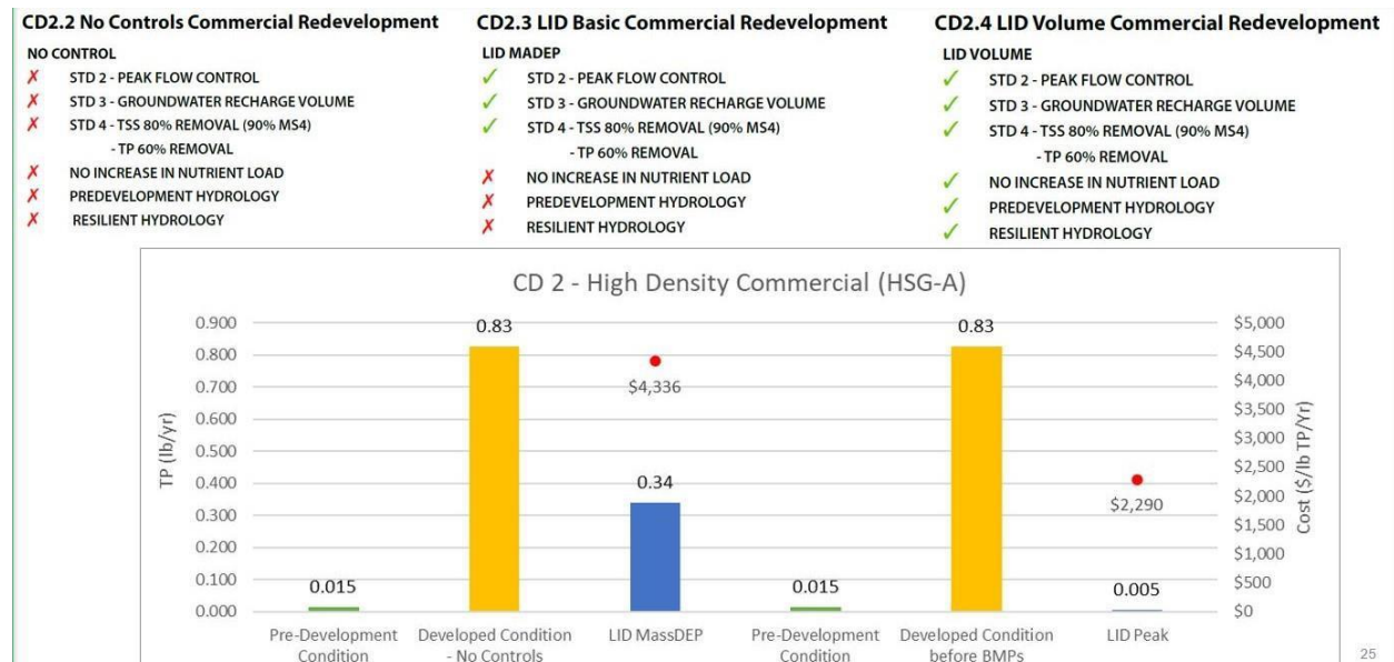
Figure 12: Water Quality Performance and Costing for CD2.3 Minimum LID and CD2.4 LID to Achieve the WPS for Commercial Redevelopment
