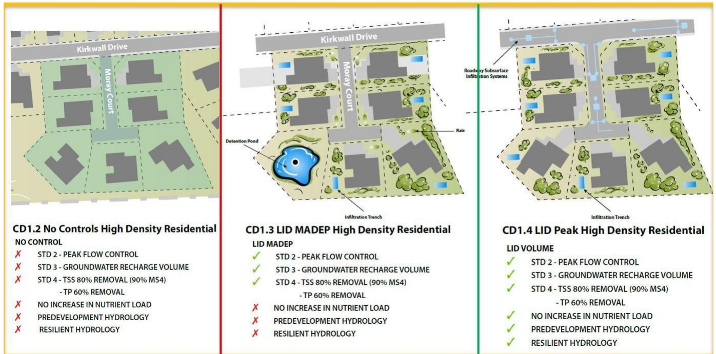
Figure 1. Concept Development Plan 1 (CD1) for High Density Residential under 3 Scenario: No Controls, Minimum LID, LID for Watershed Protection Standard
