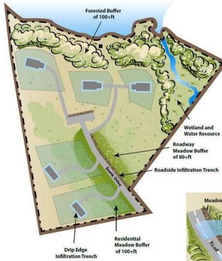
Figure 18. Concept Development CD3.4 LID to Achieve the Watershed Protection Standard for Low Density Residential
