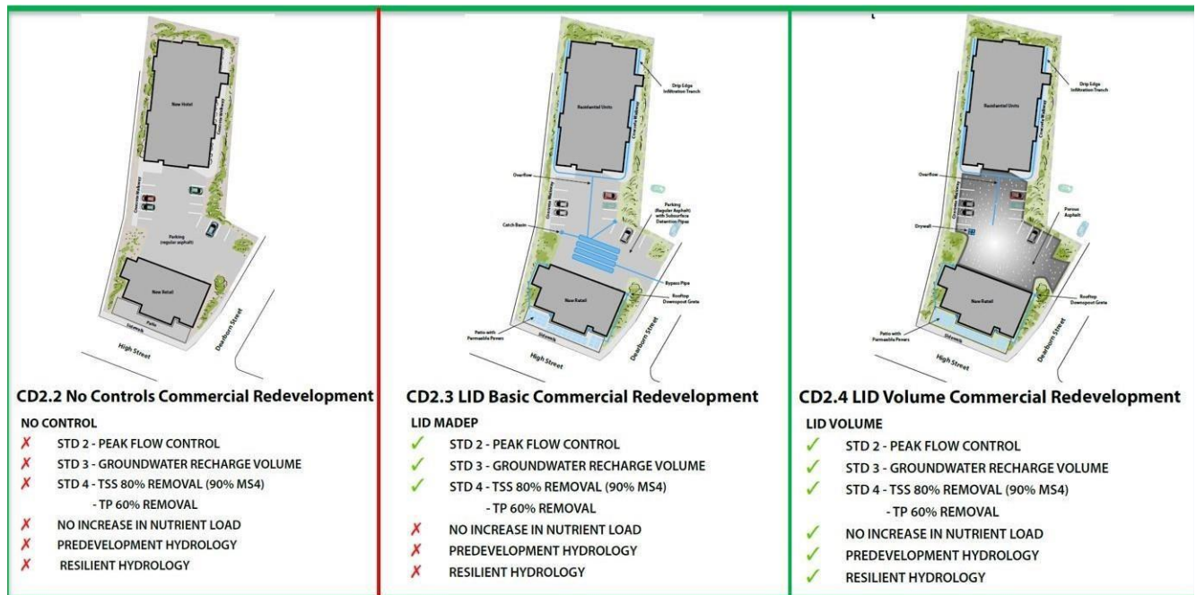
Figure 8. Concept Development Plan 2 (CD) for Commercial Redevelopment Residential under 3 Scenario: No Controls, Minimum LID, LID for Watershed Protection Standard
