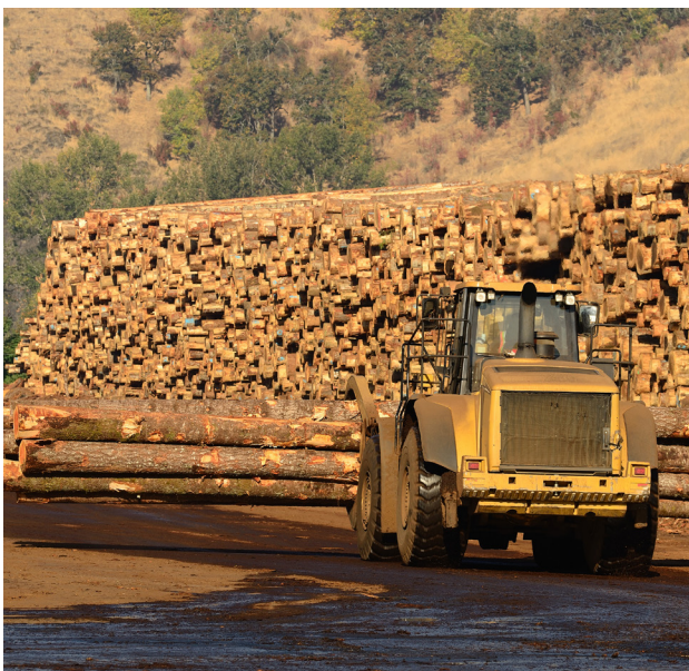
Small wheeled loader moving logs around the log yard at a local sawmill in Oregon.
