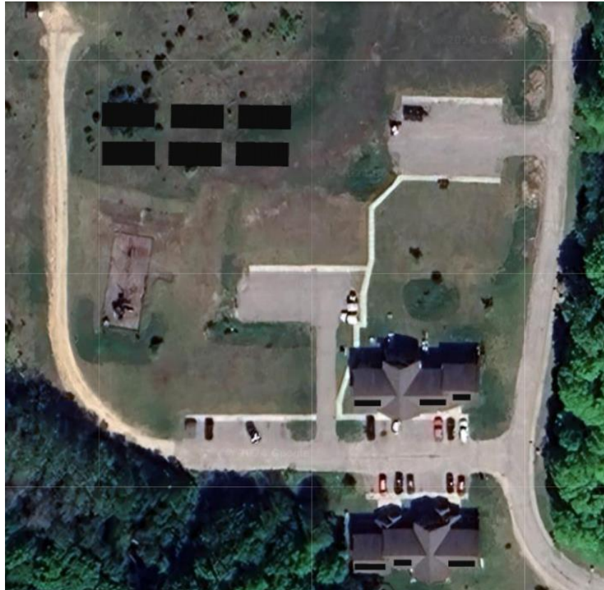
Image 1: A depiction of what the solar system at the Mtigwaakiis site could look like to offset current energy consumption after energy efficiency measures are installed (about 119 kW of solar).
