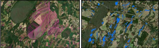
This morphology was identified systematically using shape attributes in a decision tree model. A training set of 752 features were identified as either "ditch" or "not ditch" using expert judgment. The training set was used to train a decision tree which was used to categorize millions of NWI features based on three shape attribute ratios (Figure 6-12).
