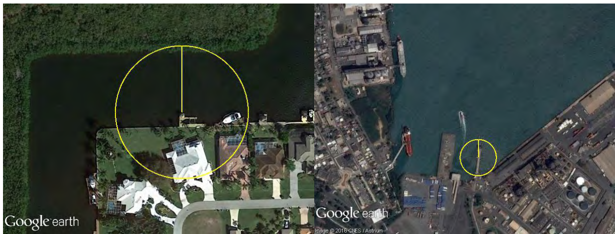
Figure 29. Example of a confined space for a noise analysis. The left image shows a 150 ft radius in a channel resulting in the channel not being wide enough to ensure more than half the channel was free from cumulative injurious noise levels. The right image shows a portion of San Juan Harbor and a 260 ft radius that would not block movement of species if piles were installed at this location because species would be able to move along the left side of the image between the 2 structures.
