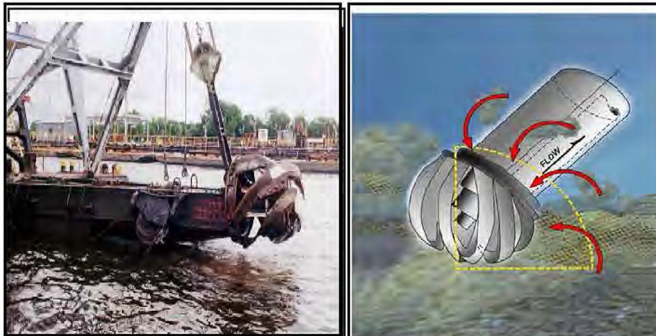
Figure 15. Cutterhead pipeline dredge schematic and representative close-up photographs (provided by USACE).
