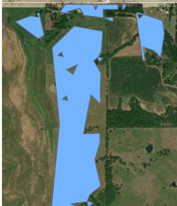
Figure 3-1. Examples of the “hole” artifact that may be generated during core map development. Holes less than 25 acres that are surrounded by areas in a core map would be added to the core map.
